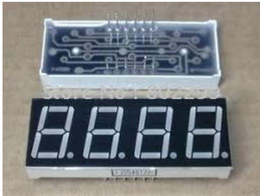
When inserting this into the board (if not already done), the decimal points should be closest to the switches/pots on the board. Line up the pins carefully, so as not to bend the pins.
